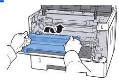
13 Return the developer unit together with the toner container to its position, aligning the guides at both ends with the slots in the machine.
